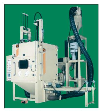
This multi-purpose shot-peening system includes an ID blast lance to peen recessed surfaces on parts, a powered loading cart, independently adjustable pressure nozzles, a shot classifier, and a combination of vertical/horizontal oscillating blast nozzles.
