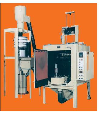
Glass-bead system for peening jet-engine turbine blades incorporates vertically oscillating nozzles, a vibratory bead classifier, and one rotating work station.
