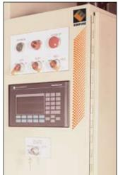
Interface terminal enables operator to designate blasting parameters such as nozzle stroke length and oscillation speeds, ON/OFF status of selected nozzles, part rotation speeds, and blast duration by simply inputting the appropriate part identification number.
