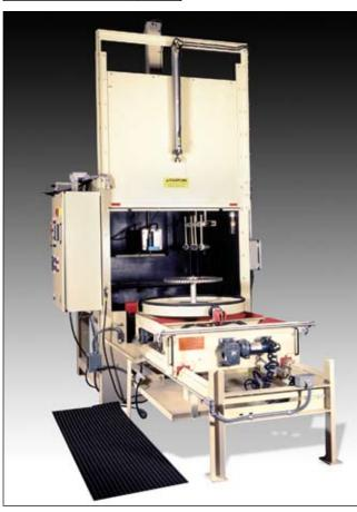
Versatile peening machine enabled a repair center for jet-engine parts to expand its business into the areas of disc and hub rebuilds. In addition to peening recessed surfaces, the unit processes many different size parts ranging up to thirty inches in diameter.
