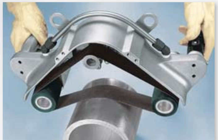
14300 Dynangle® II accepts abrasive belts 2" wide by 34" long (51 mm x 864 mm), effective for slack polishing of cylindrical surfaces up to 36" (914 mm) in diameter. This machine is also great for surface conditioning on flat surfaces, using optional platen accessory.
