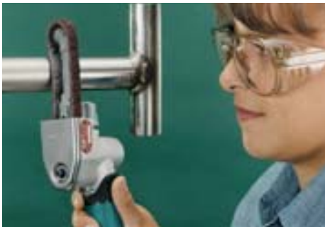
Clean and finish using non-woven nylon belts.
