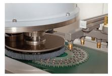
For powder metal applications, either green or sintered, parts are flipped automatically for streamlined deburring — both sides in a single pass!
