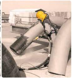
GMA Garnet<sup>™</sup> consists of totally natural almandine garnet known for its natural hardness, durability and abrasive characteristics. It is free of any heavy metals or toxic components and meets all Occupational Health & Safety requirements.
