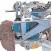
The central head carrying the tools is an extremely strong and compact unit. The gear head is mounted in an ingenious, unique scissortype suspension system. The strong design allows transmission of high torque values through the 6 conical spindles.
