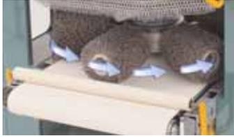
The gearing of the spindles vary between the pairs to ensure uniform finishing of all faces on the parts and uniform wear on the finishing tools.
