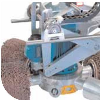
The central head carrying the tools is an extremely strong and compact unit. The gear head is mounted in an ingenious, unique scissor-type suspension system. The strong design allows transmission of high torque values through the 6 conical spindles.
