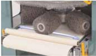
During the process, the entire head and the six spindles rotate and oscillate across the surface of the parts, which means that the processing of the surface is applied from every possible direction, no matter how the part is placed on the conveyor or belt.
