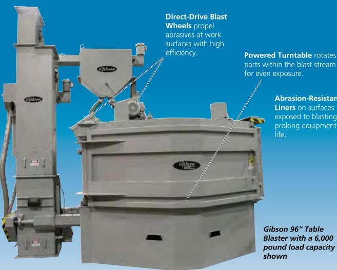
**Abrasion-Resistant Liners** on surfaces exposed to blasting prolong equipment
