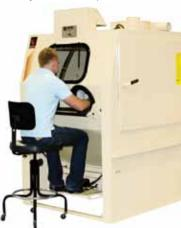
Designed for sit-down blasting, these ergonomic cabinets include a padded armrest, an elevated foot rest for treadle control, top-entry piping for less arm stress, a sound dampener to reduce noise and a front mounted pressure regulator — all aimed at improving operator comfort and performance during long, repetitive blast cycles.
